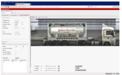
The video system detects vehicle registration numbers, container codes (ILU and BIC codes) as well as hazardous goods and waste labels. A careful selection of state-of-the-art sensors is used for this purpose. The separation of vehicles and loading units is achieved with special 3D cameras and a continuous adaptation of our Numberfinder software.
